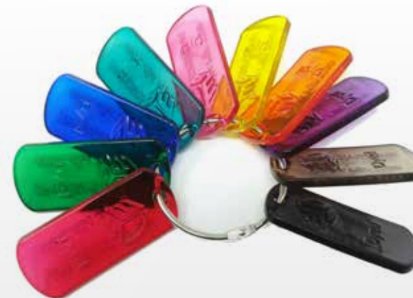
Visijet M2R-CL color keyring with clear coating dyed with standard colors with 1% concentration (60 °C and 30 min)
