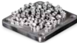
Partials, copings and bridges production in LaserForm CoCr (B)
