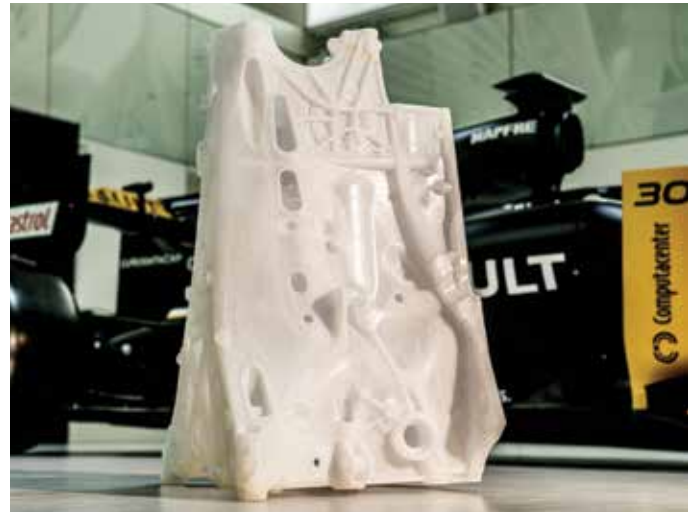
3D printed investment casting patterns provide accelerated access to large, high complexity metal parts.
